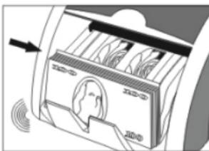
**NOTE:** Because the machine stops unconventionally, it may lead in miscarriage of detecting the next banknote, so you must re-count these banknotes.
