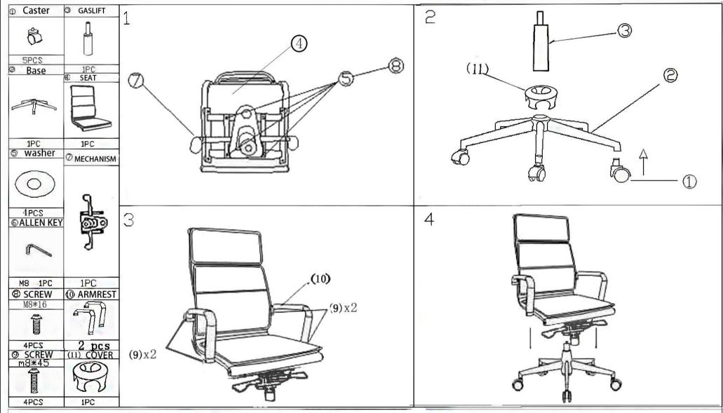
It is important to assemble all parts as the direction ARROWS point to. Make certain that all screws are fully tightened before using the chair, Each month check all screws and tighten those my loose. WARNING:Do not stand on the chair for any purpose.
