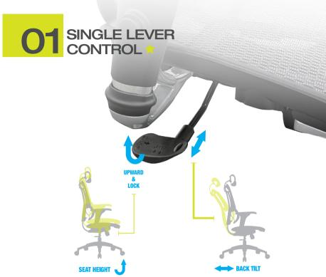
Lift the lever up J and hold to raise or lower seat height. Release the lever to lock seat height.
