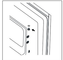
7. Rotate freezer door and place hinge side at left side. And then fix the door by holder.
